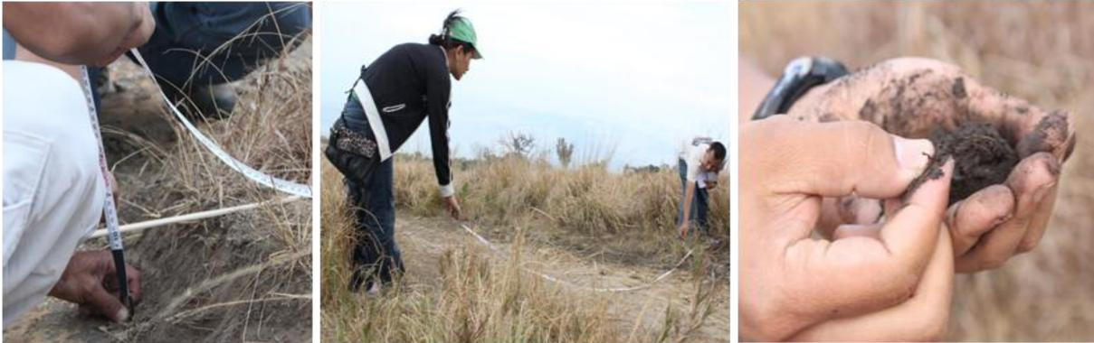
Figures 2-4. Measuring depth of soil, width of damage sustained by vehicles and texturing soil.
